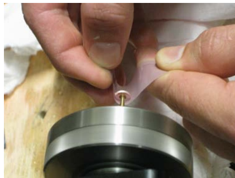
Figure 13: Wrapping Diamond Sandpaper
