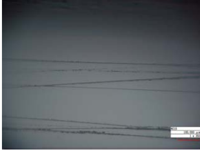
Figure 6: Gouges Due to Aluminum Oxide Residue
