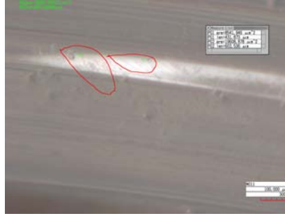
Figure 7: Surface Imperfections Due to a Fingerpad
