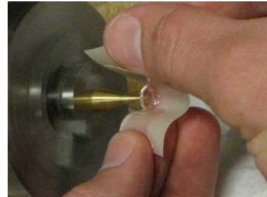
Figure 5: Polishing on Lathe by Hand
