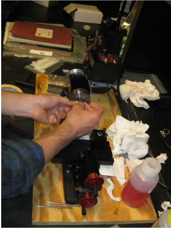
Figure 11: Polishing on the Mini-Lathe
