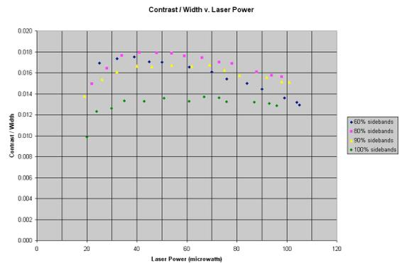
Figure 10: Contrast/width versus laser power.
