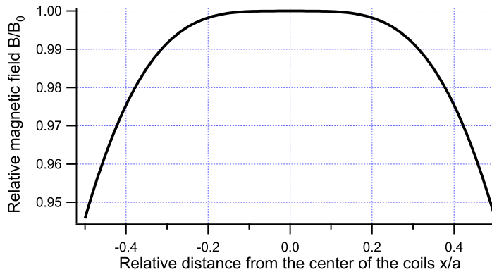
Figure 4: Dependence of the magnetic field produced by a Helmholtz coil pair B of the distance from the center (on-axis) x/a . The magnetic field is normalized to the value B_0 in the center.
